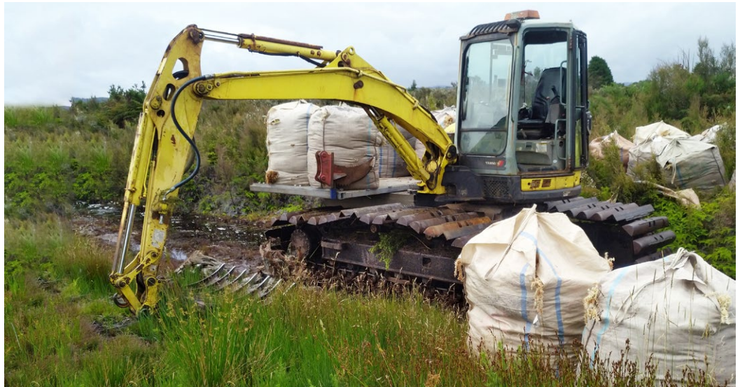
Bruce’s one-of-a kind-digger, a 22-tonne track base with Yanmah ViO5.5 tonne top, complete with tipping deck on the back. It was all put together at Dispatch Engineering in Greymouth, and carted by T Croft Ltd.
