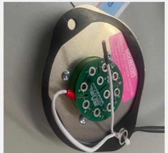
Pic3 – PCB inside the Civacon plug
