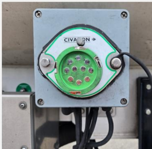
Pic1 – Civacon branded “green face” plug on fuel tanker
