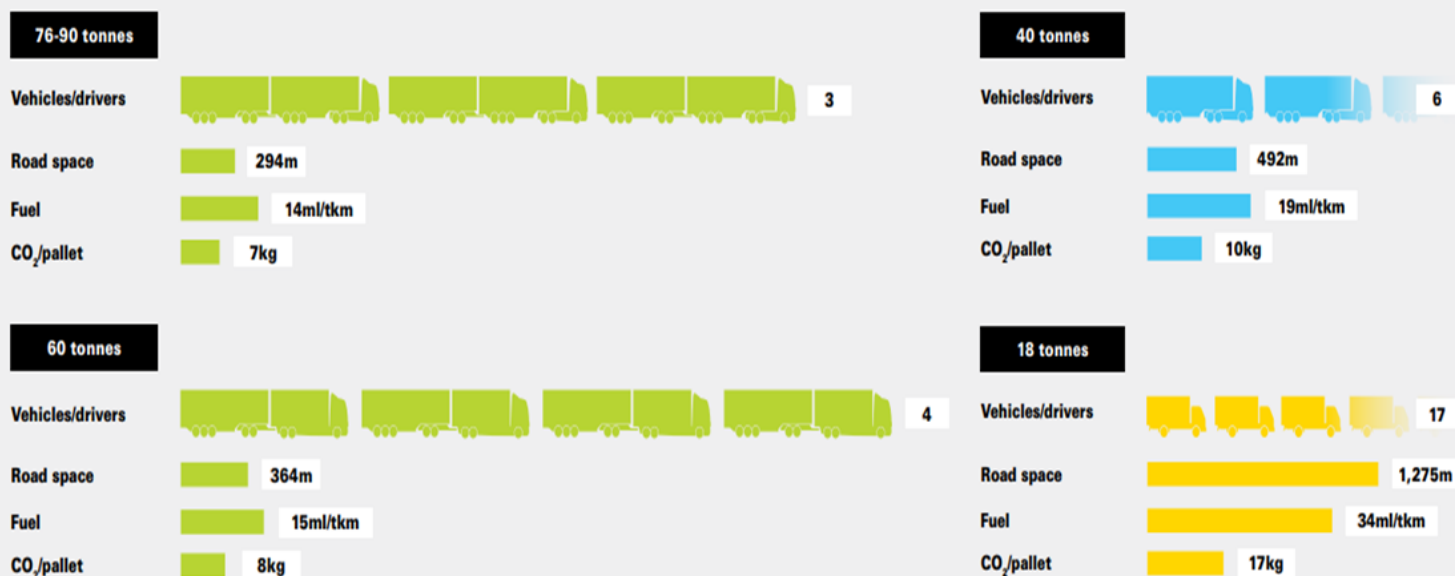
Number of vehicles, road space, fuel and CO 2 emissions for a 200-pallet load (source: IRU)
