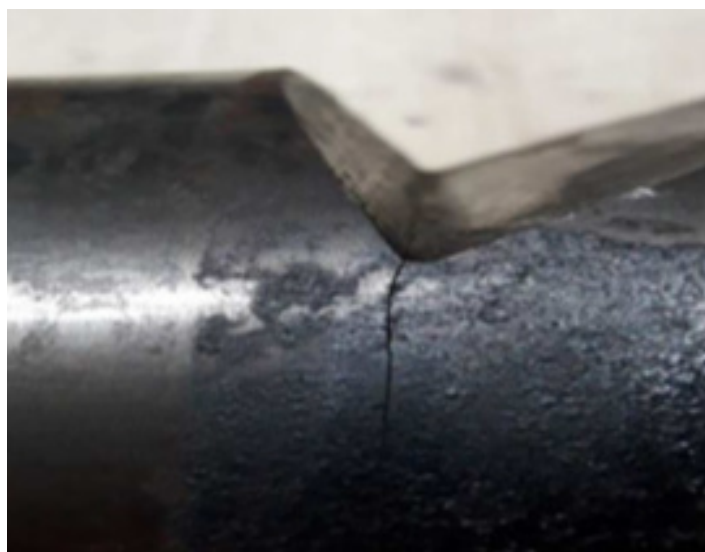
Figure 6: Substandard pin (source NZ Police)
